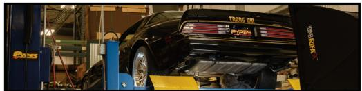
1. Begin by placing the vehicle on a lift or four jack stands at maximum height to aid in an easier installation. To help ease the installation, pre-fit all the components into a complete system on your garage floor, using the diagram provided.
